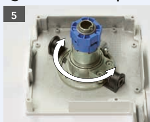
Roughly align the gearbox in the direction of the drive rod (45° or 90°)
