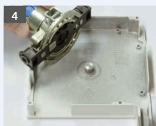
Fit the bevel gearbox with quick-fit system and clamping plate onto the shortened trunnion.
