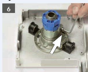
Tighten the screw on the clamping plate (can be screwed on both sides) using a 3 mm Allen key.
